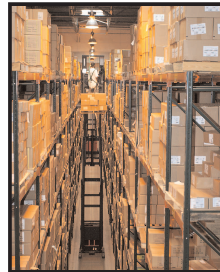
Tethered by a safety strap, a VHPS employee uses a forklift to gingerly lower a pallet load of books from three stories up at the 450,000 square foot book distribution and warehousing facility. Note the wire guidance system in the floor that keeps the fork lift centered in the aisle.
