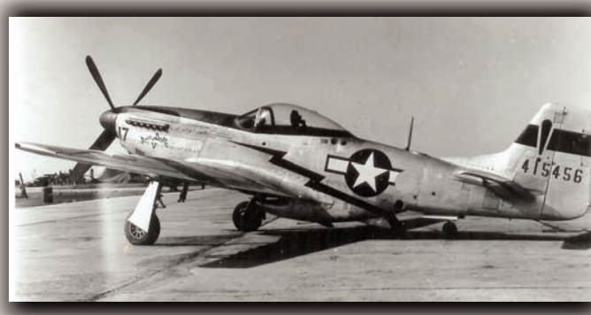
Below, the P-51D with its trademark bubble canopy packed quite a punch: six 50-caliber machine guns, two 500-pound bombs or two napalm bombs, even rocket launchers. With external tanks, the plane could fly eight hours straight. Japanese "Oscars" were no match for this deadly force.
