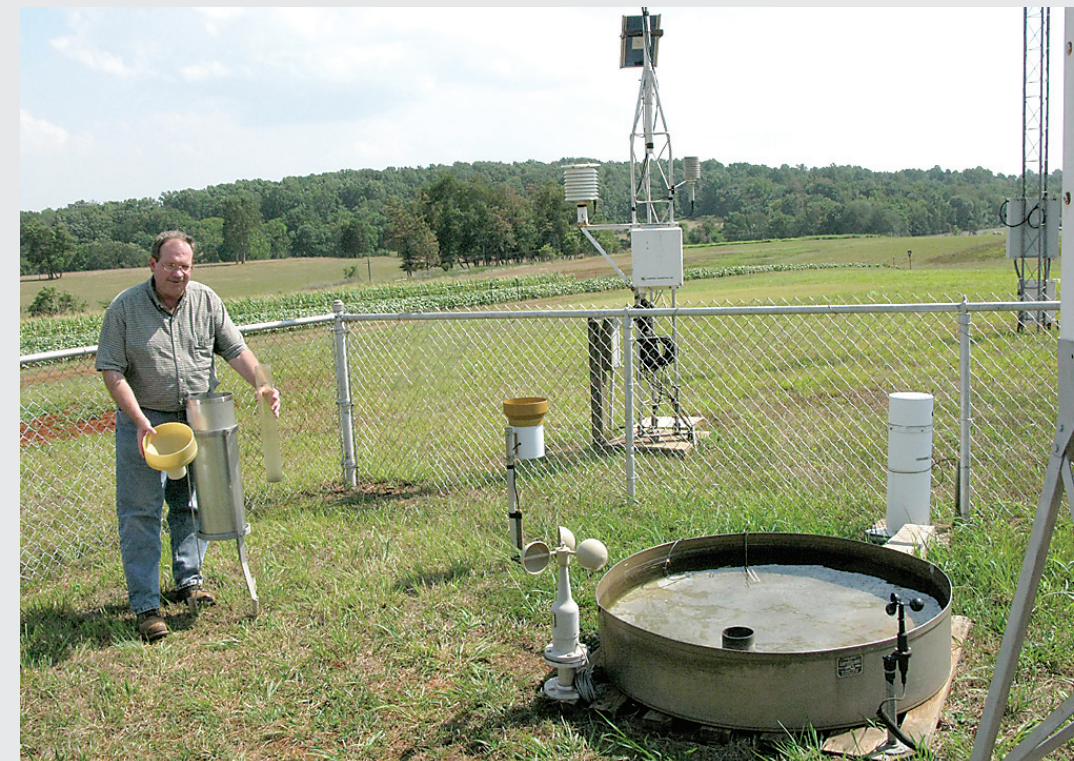
Every day since 1941, official weather data has been recorded at the Northern Piedmont Agricultural Research Station outside of Orange. In the right foreground is the pan that measures evapotranspiration. To the left, station superintendent Dave Starner demonstrates the official rain gauge that has recorded precious little moisture over the past three months. In the background, that thing that looks like a stack of white pancakes is the thermometer that has recorded record-breaking heat this summer.
