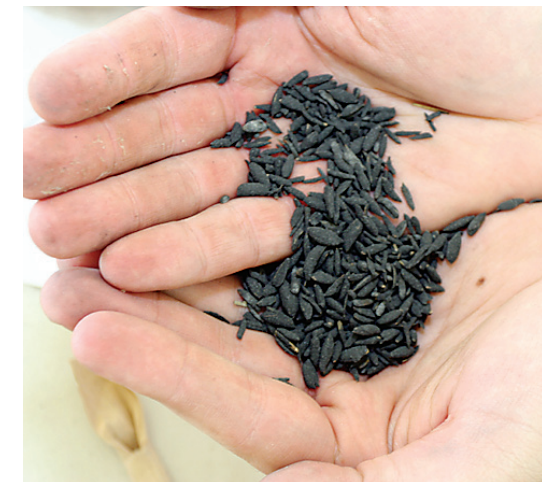
Sometimes the bursting charge consists of black powder coated rice hulls.
