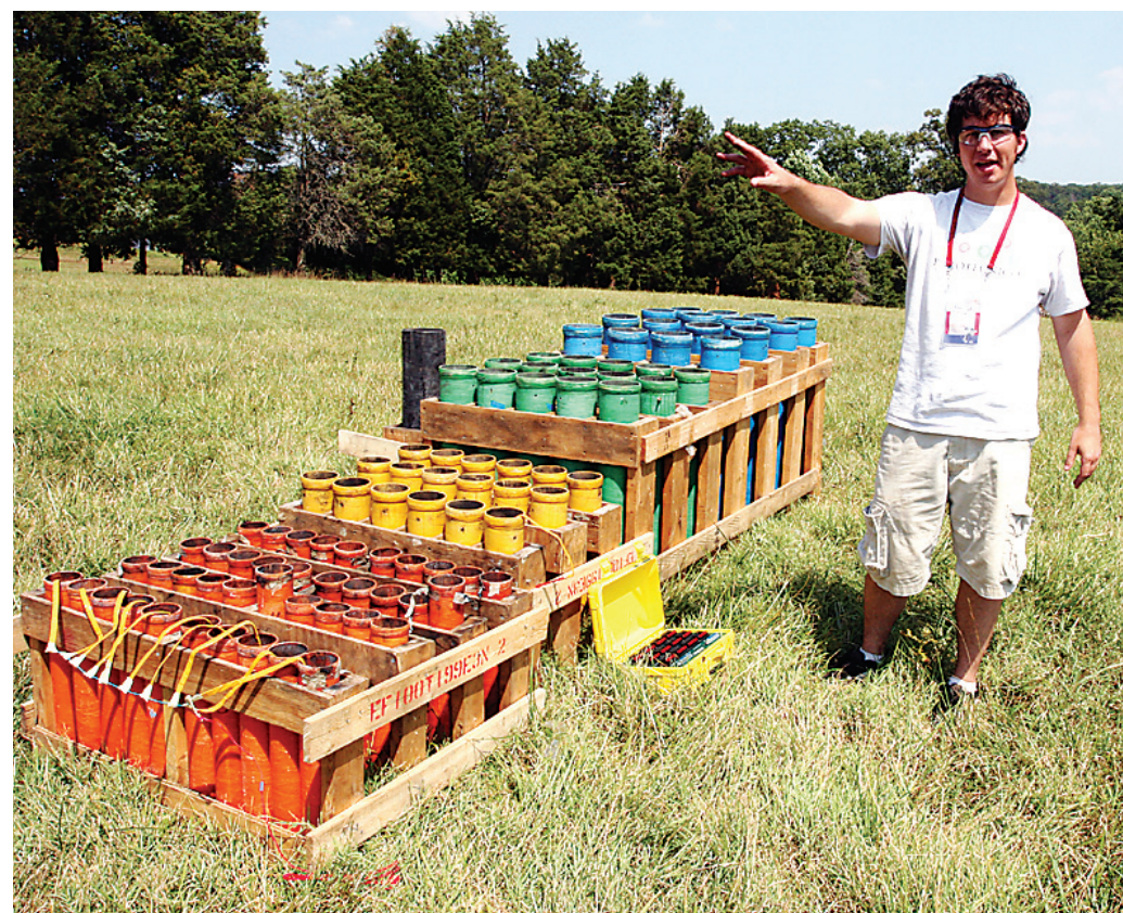
Above, Crackerjacks Vice President George Tasick shows how mortars are arranged in a pod. They can be fired remotely through the electric firing box at his feet. Top photos, Examples of the Rocket Man, Tom Rebenklau's artistry.
