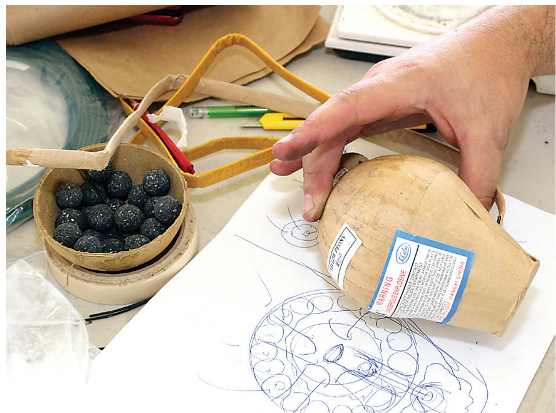
Basic ball shell construction. Note the stars in the hemisphere that surround the bursting charge which ignites via a pass fire from the lifting charge that sends the shell up into the air.
