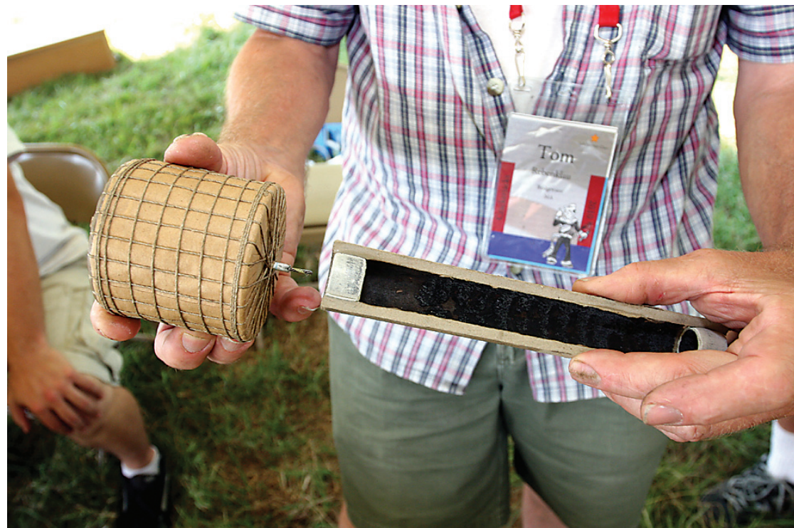
The inner workings of a Tom Rebenklau rocket. Powder is packed around a spindle in the cylinder to make the rocket motor. The painstakingly constructed canister on top contains the multicolored burst.
