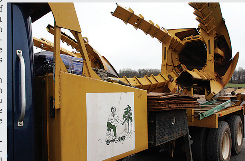
PHOTO BY PHIL AUDIBERT Grelen has two tree spades. One can dig a 65-inch ball; the other a 90-inch ball. The machines make it possible to plant trees 30 and 40 feet high.
