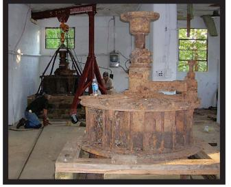
Photos courtesy Kevin O'Brien and Rapidan Renewable Energy and FPC Before and after: an original 1930s-era turbine before being shipped to the Leffel factory in North Carolina, and the same turbine after refurbishment.
