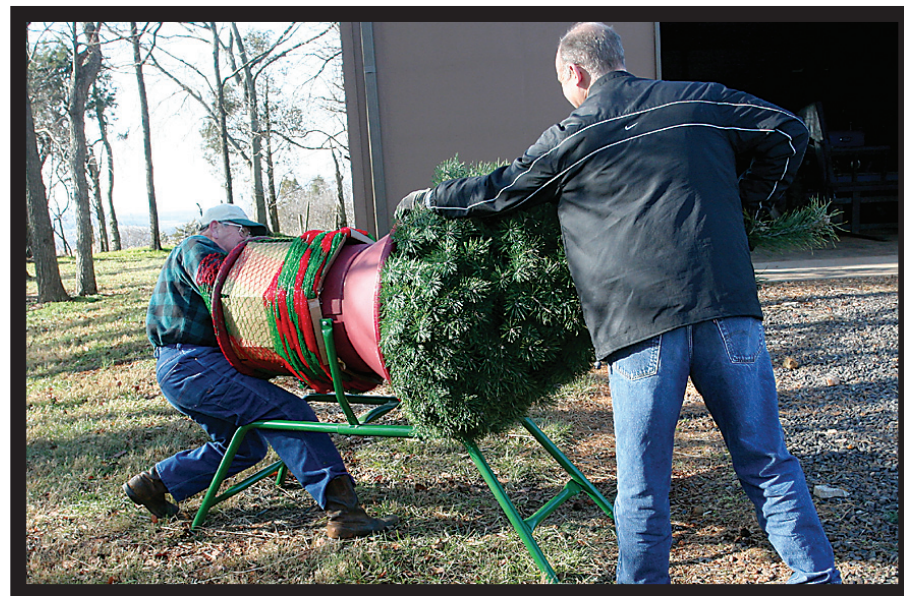
Steve Satterfield (left) tugs a Christmas tree through a device that binds the branches in red and white netting. The netting protects the tree from wind damage on the ride home.
