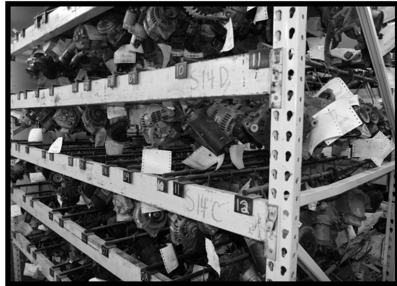
Every part removed from the car is tagged with a number that tells the source of the part and its exact location by building, row, shelf and slot.
