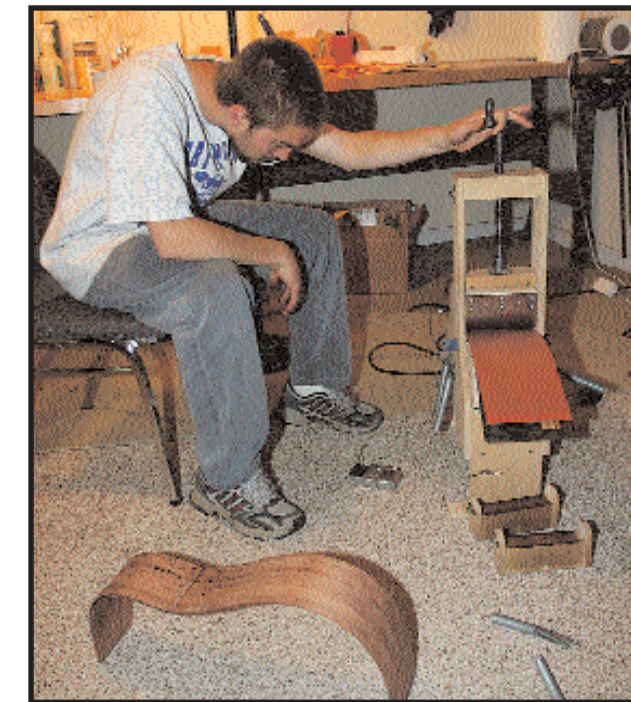
Above, although these particular examples will not be used, they show the bracing patterns for guitar tops and backs. Bracing plays a crucial role in how a guitar sounds. Below, Adam McNeil gradually cranks down on the waist of some guitar binding that he is shaping. Note the completed half side in the foreground. The process of wetting and heating the wood to bend it into a guitar side has drawn sap to the surface. It will be scraped and sanded away before finishing. Photos by Phil Audibert
