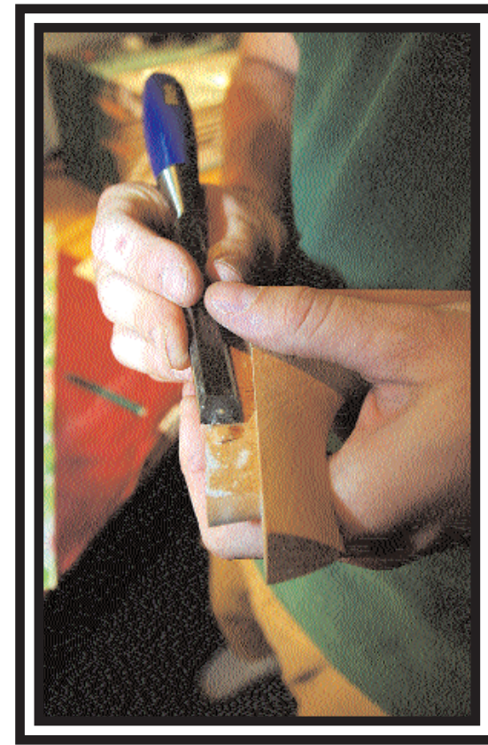
Above left, Brian Calhoun uses a tiny coping saw such as this to cut each piece of inlay. Not only does he do this work for all Rockbridge guitars but also for high-end Stelling banjos. Above right, using "blazing sharp" chisels, Brian Calhoun makes minute adjustments to the dovetailed neck joint. Although certain routine tasks are done by machines, the most delicate are accomplished with hand tools. Below, that's a Rockbridge guitar that Rhonda Vincent is playing. The bluegrass artist owns three. Top photos by Phil Audibert. Bottom photo contributed.
