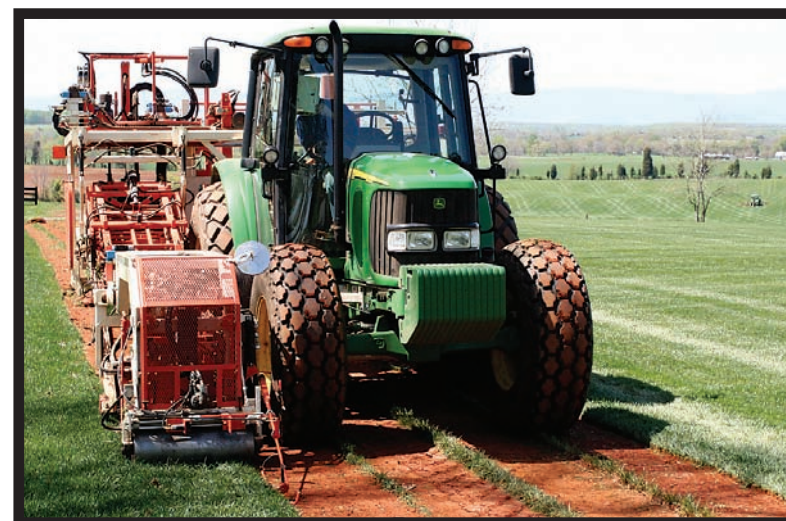
Photo by Phil Audibert William Scott operates the sod-cutting machine at Somerset Seed and Sod's Jacksonville area farm as another employee mows established turfgrass in the background. Note the checkerboard pattern left by the 22-foot rotary mower.
